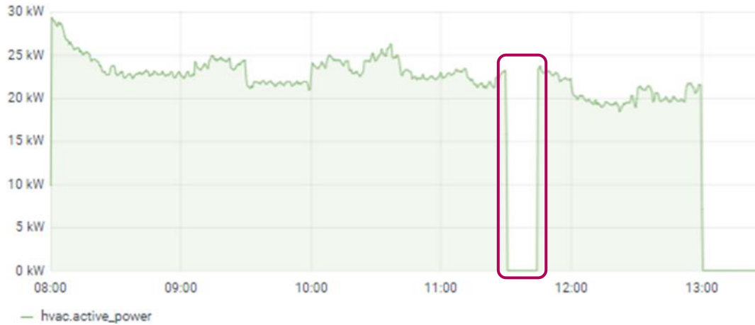
Figure 44 HVAC control activation signal sent by the aggregator to Tabacalera Polo Digital sFSP
